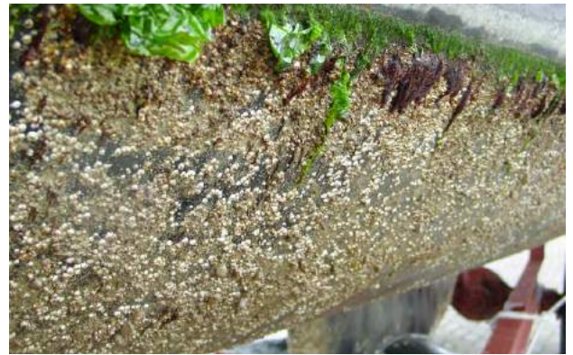
Macrofouling on a motor vessel
