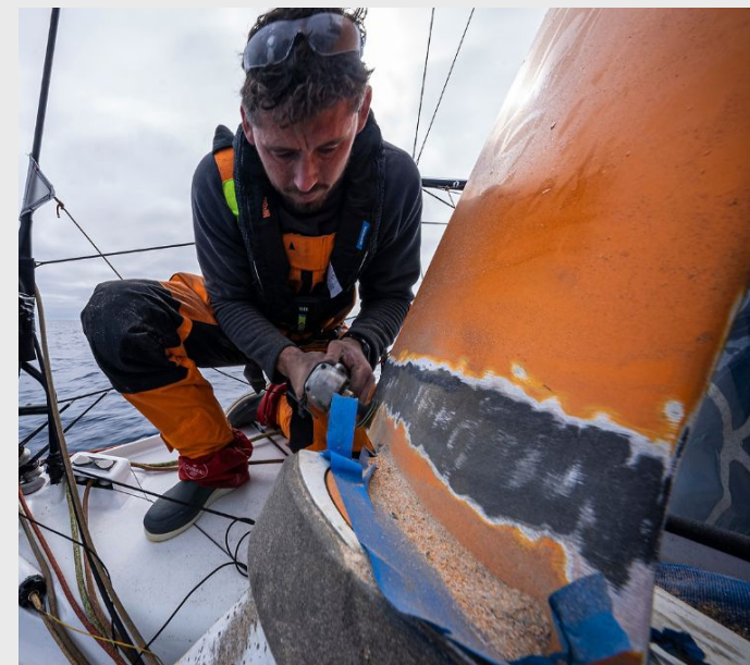
Image: Fixing a damaged rudder
