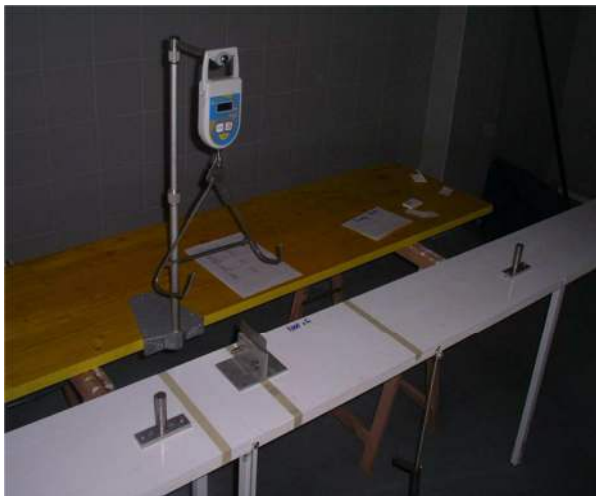
Mast weight / centre of gravity (left) and tip weight (right) measurement. The centre of gravity may be checked using a knife-edge to balance the mast.
