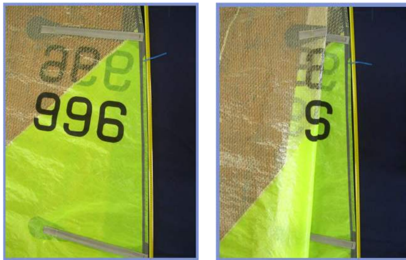
Figure G.2.3.3 Leech hollow before and after flaking.
