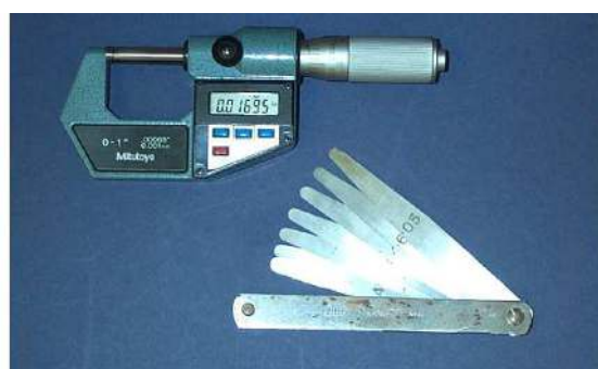
Figure G.1.2.3 A digital micrometre of resolution 0.001 mm and feeler gauges for sail cloth thickness measurement
