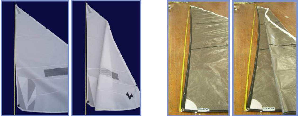
Figures G.2.3.1 & G.2.3.2 Leech flattening before and after flaking.
