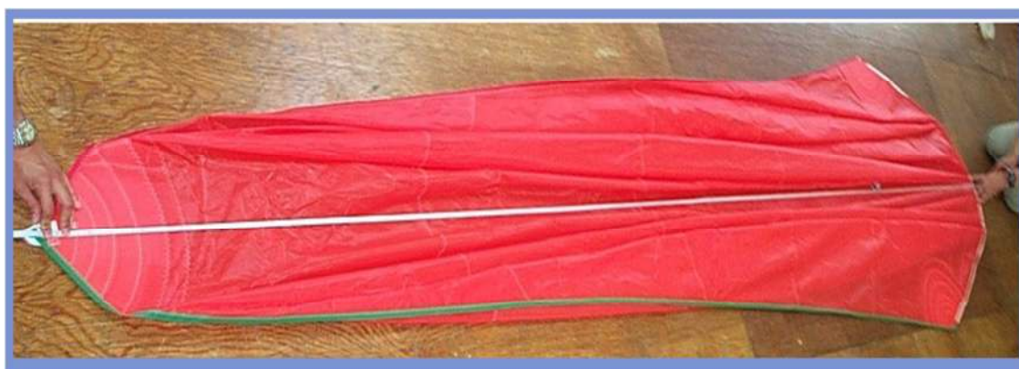
Figure G.2.3.7 Spinnaker foot median.
