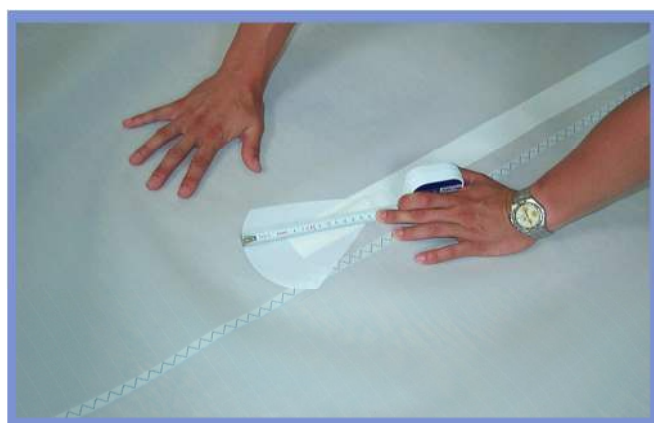
Figure G.2.4.3 Batten pocket patch size.
