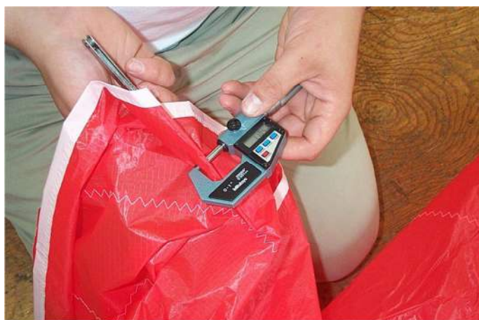
Figure G.1.2.3 Ply thickness measurement using a micrometre and feeler set.
