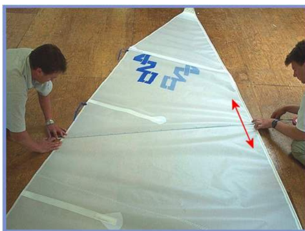
Figure G.2.3.8 Mainsail half width.
