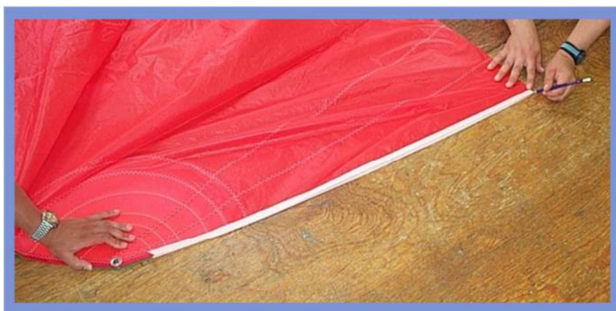
Figure G.2.2.3 Spinnaker mid foot point.
