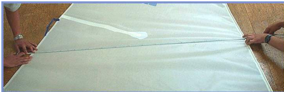
Figure G.2.3.4 Proper tensioning of sail for wrinkle removal; when wrinkles are formed parallel to the line of measurement the tension must be relaxed.
