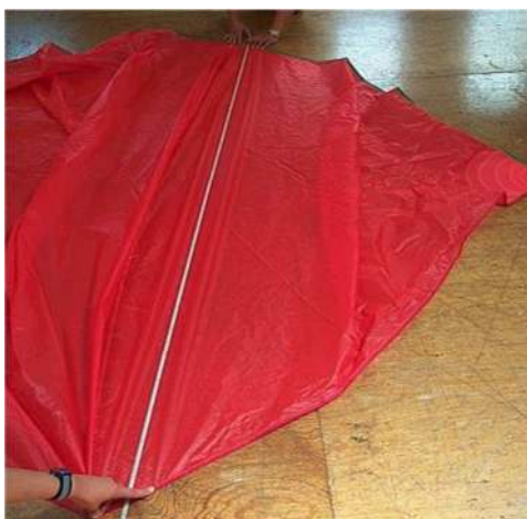
Figure G.2.3.10 Spinnaker half width.
