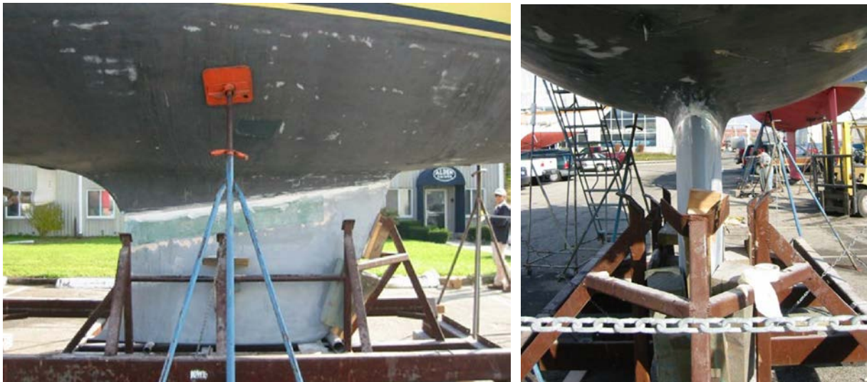
FIGURE 4 – Note the tight fit of the replacement keel to the existing keel stub.
