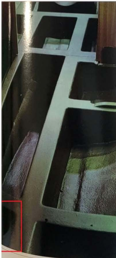
FIGURE 5 – Photo from Ferenc Mate's The World's Best Sailboats featuring the Sweden 41 with its innovative molded hull bottom framing grid. This photo shows a Sweden 41 under construction and shows the grid and keel root from forward looking aft. The red box indicates the location of the recess in which the mast step would later be installed. To the right is a depiction of a "hat section" and a photo of Gunga Din's mast step recessed in the cavity.
