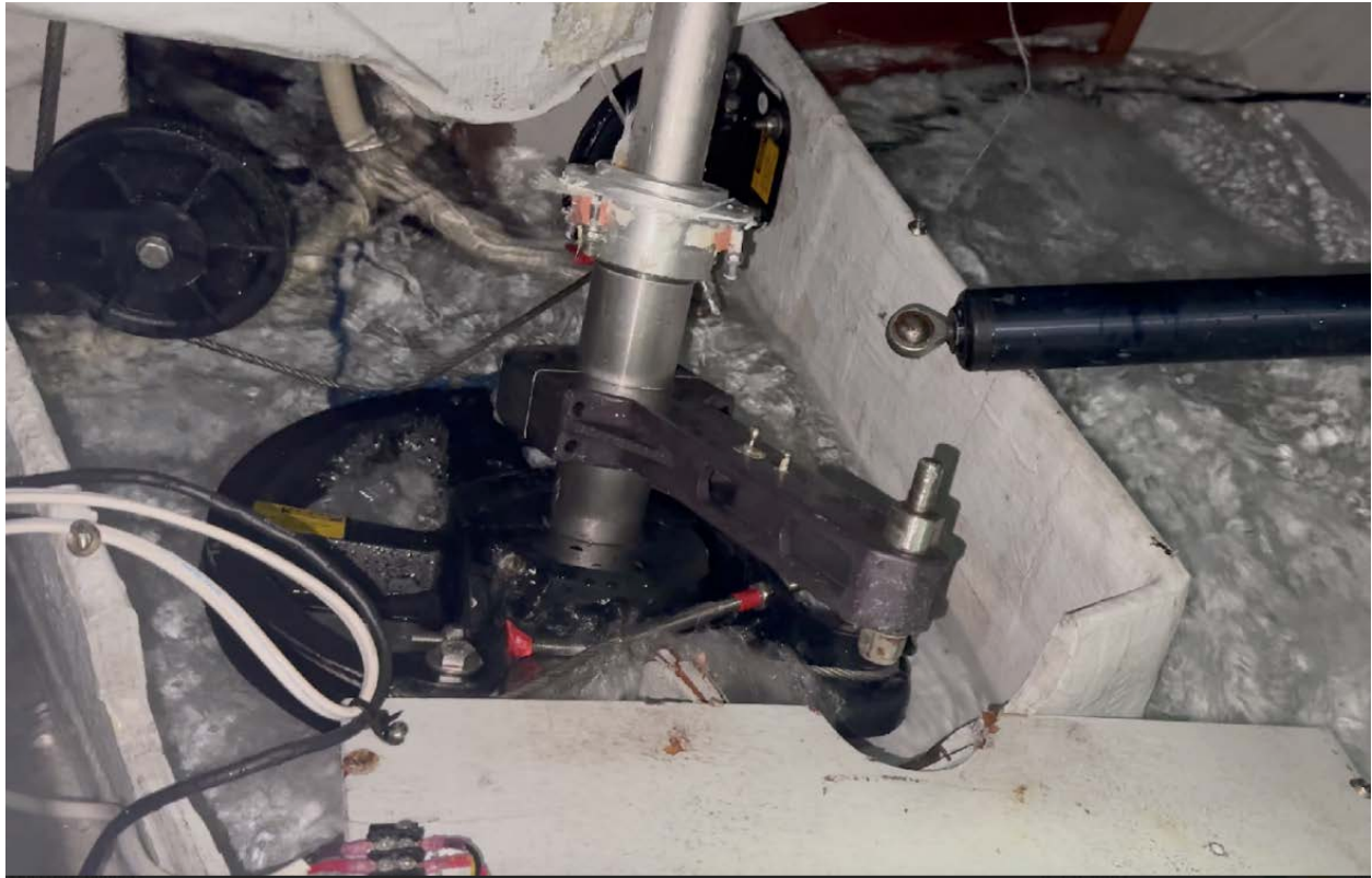
Figure 1 This picture, taken approximately 40 minutes after the incident, shows the damage and flooding to Alliance. The upper rudder bearing is visible mid-picture above the autopilot tiller arm, having slid down the rudder stock from its original position in the cockpit sole.
