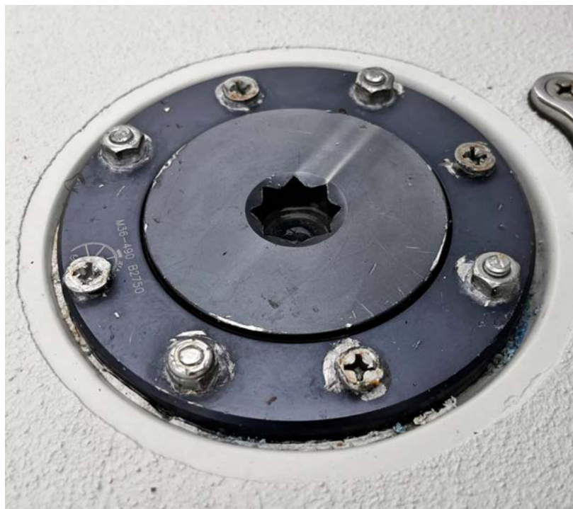
Figure 9 The repaired bearing aboard Ceilidh .
